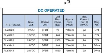
When soldering the relay to the PC board, solder temperature must not exceed +270°C, and solder time must not exceed 5 seconds. If necessary to hold the relay in place during soldering, the terminals of the coil and movable contact arm may be slightly bent after insertion through the board holes.
