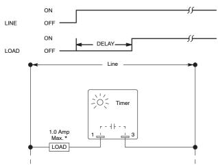
\* For higher current applications connect a switching relay in series with timer in place of load
