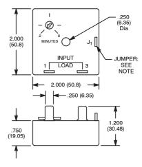
NOTE: 18-40 V AC or DC Cut J<sub>1</sub> for 40-264 V AC, DC
