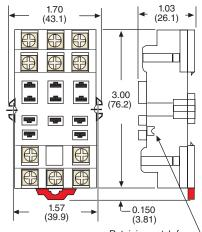
Retaining notch for hold down clip (2 Places)
