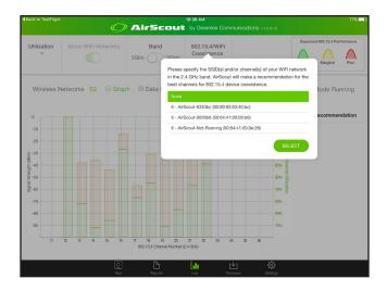
Once a network is selected, 802.15.4 recommended channels are displayed on the right that correlate with the small parabolas on the bottom of the graph. Parabolas marked in green are the current best suggested 802.15.4 channels, with red being the worst. The resulting channel plot can be used to tune 802.15.4 networks by setting frequency hopping masks that correspond to these best channels while avoiding interference or congestion from other channels.
